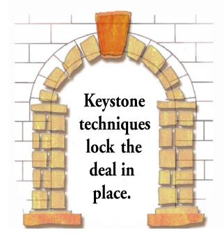
What made ancient Roman temples, aqueducts and bridge structures stand the test of time was the contour and balance of the Roman arch. The strength of the Roman arch is based on a single, specially-shaped stone – the Keystone, that locks everything into place.
